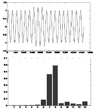
Fig: 3(c): Sine wave with voltage swell and its energy distribution diagram
