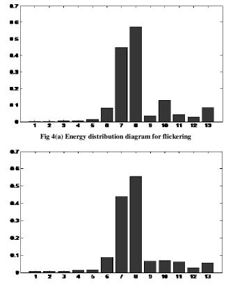
Fig 4(a) Energy distribution diagram for capacitor switching
