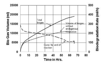
Fig. 1. Evolution overtime of the volume of biogas produced, of the volume of biogas withoutendogenous respiration and of the curve used to identify the end of the reaction (Biogasactivity curve, fruit substrate)
