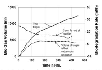
Fig. 3. Evolution overtime of the volume of biogas produced, of the volume of biogas without endogenous respiration and of the curve used to identify the end of the reaction (Biogas activity curve, Oil substrate)
