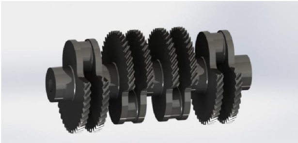
Figure.2.4.1. shows the new design of the crankshaft along with the relief bores and geared section
