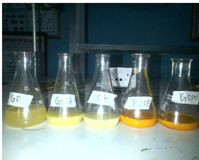
Plate 1. Picture of the biodiesel produced; from left to right GO, GOCF, CF, POCF and GOPO
