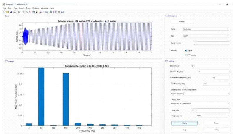
Fig. 11. Total Harmonic Distortion(THD) in the P&O Technique
