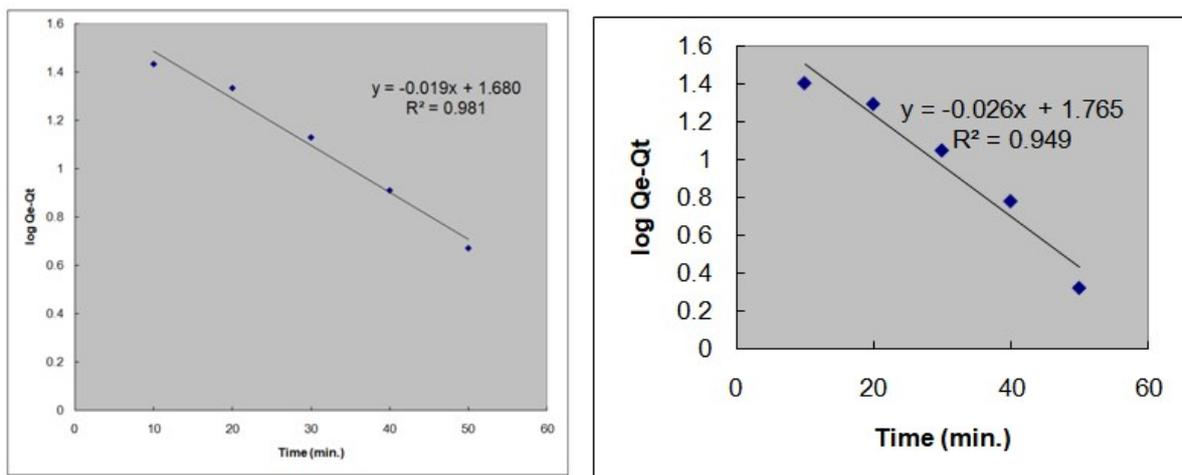
Figure 6. Fit of pseudo first order kinetics for MB dye adsorption on both (A) phosphoric acid and (B) KOH based activated carbon
