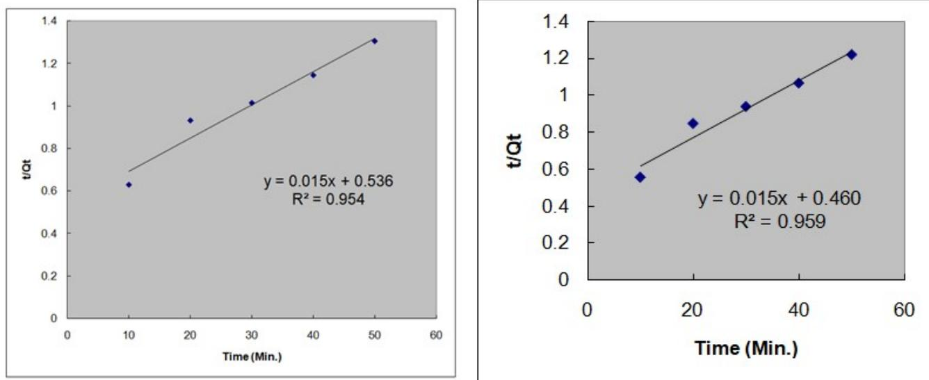
Figure 7. Fit of pseudo second order kinetics for MB dye adsorption on both (A) phosphoric acid and (B) KOH based activated carbon
