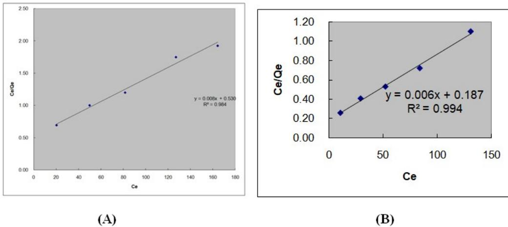
Figure 4. Correlation graph for Langmuir isotherm for adsorbent impregnated with (A) phosphoric acid and (B) KOH
