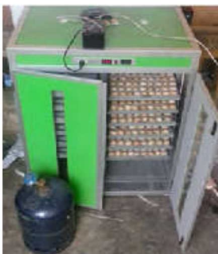
Figure 3. Incubator operating with a 12 or 24V photovoltaic system
