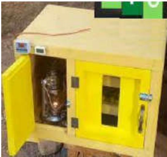
Figure 2. Incubator operating with a petrol lamp
