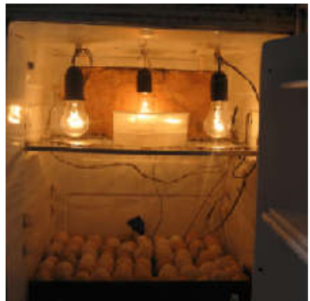
Figure 6. Incubator incorporated with incandescent lamps
