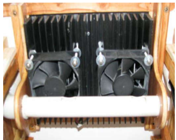
Figure 5. Built-in incubator with heating resistors
