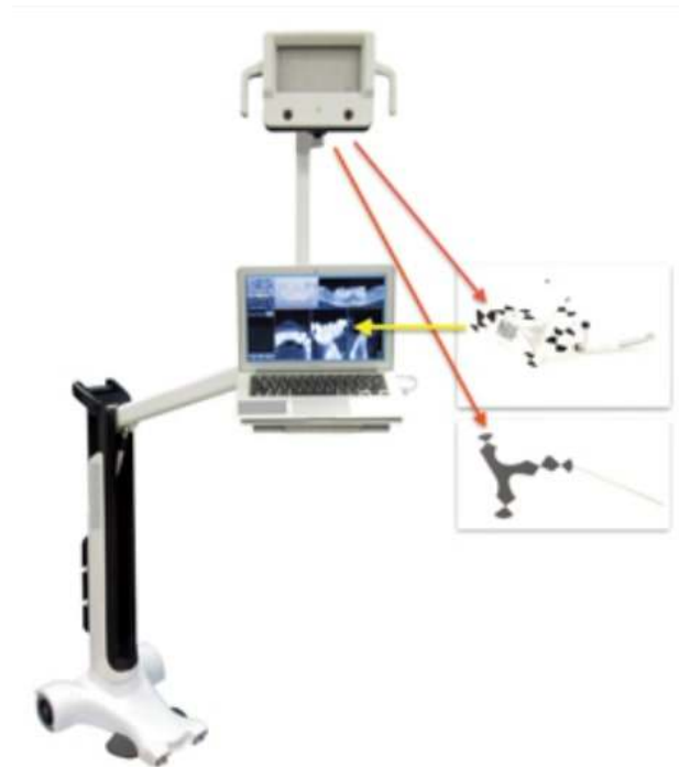
Fig. 1. An optical tracking sensor tracks the JawTracker, Tracer-Tracker, Drill-Tracker and instrument. (Courtesy: Dr. Kenneth S. Serota)
