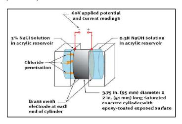
Figure 6. Rapid Chloride Ion Permeability Apparatus
