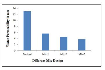
Figure 5. Water permeability of different mixes
