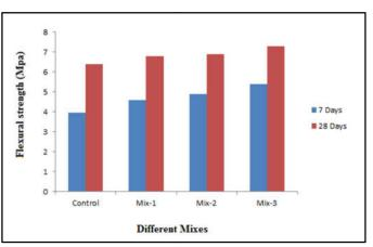
Figure 4. Flexural strength of different Mixes
