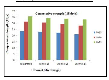
Figure 2. Compressive strength of 28 Days (Different Mixes)
