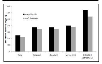
Figure 5. Effect of treatments on dry crease recovery angle (Warp and Weft Directions)
