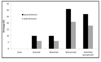
Figure 3. Effect of treatments on fabric sett (Warp and Weft Directions)
