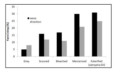
Figure 1. Effect of treatments on yarn crimp (Warp and Weft directions)
