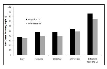
Figure 6. Effect of treatments on wet crease recovery angle (Warp and Weft Directions)
