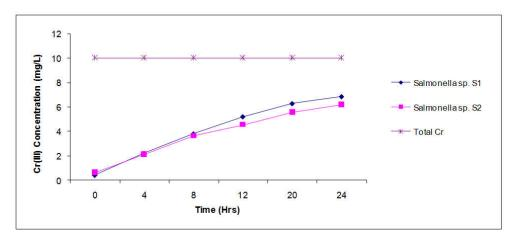
Fig. 8. Quantification of total chromium and Cr(III) during optimization of temperature
