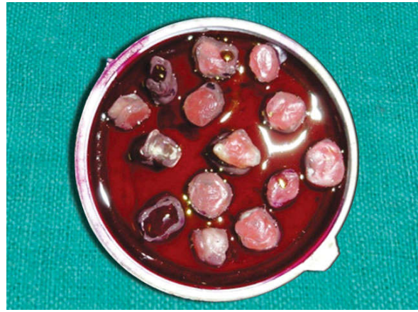
Figure 6. Restored samples dipped in Basic Fuchsin dye
