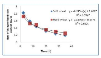
Fig. 2. Rate of change of moisture content with respect to time
