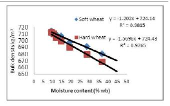
Fig. 1.Effect of moisture content on bulk density of soft
