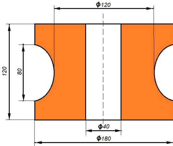
Fig. 2. Drawing of a roller used for FEM calculations
