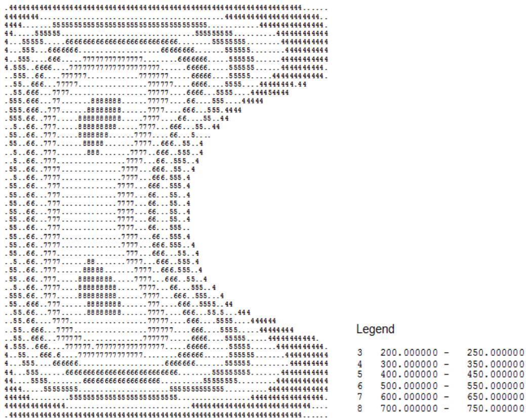
**Fig. 4. Temperature field in °K in the roller (see Fig. 2) at the moment 50 sec when direct convection quenching with heat transfer coefficient equal 10,000 W/m<sup>2</sup>K**
