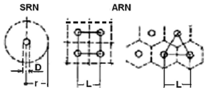
**Fig. 1. Positions of round holes in the sprayer used for intensive quenching of large steel part**
