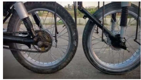
Fig.10. 2 nd and 3 rd wheel arrangement view
