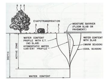
Figure 2. Water content profiles in the active zone (Nelson and Miller, 1992)
