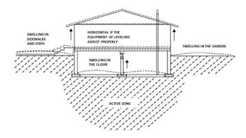
Figure 2. Ground movement associated to the construction of a shallow foundation over an expansive soil (Fredlund and Rahardjo, 1993)
