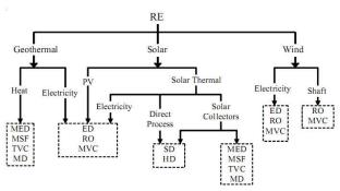
Fig1. Technological Combinations of Conjunction of Renewable Energy with Water Purification Technologies
