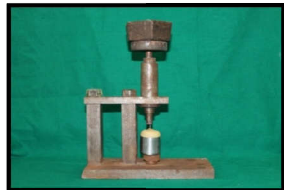
Figure 3. Special tray with impression material in die orientation apparatus
