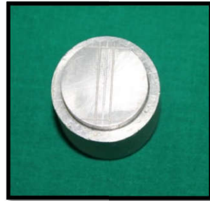
Figure 2. ADA specification no.19 master die
