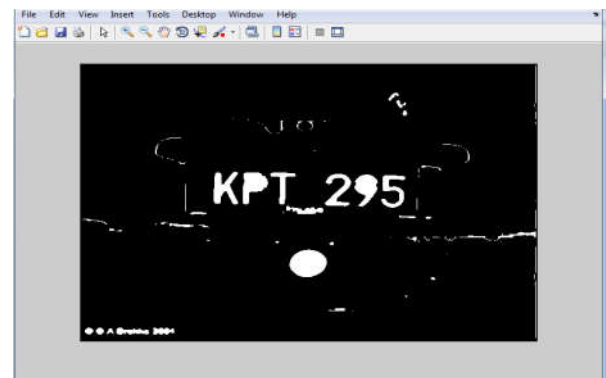
Figure 7. Erosion Using Line As Structural Element
