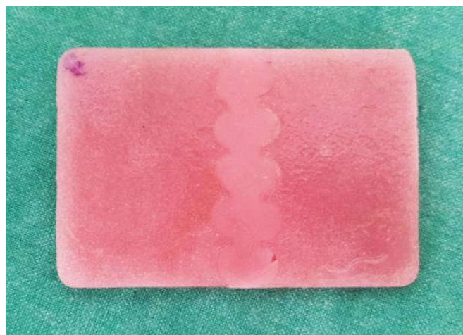
Fig.5. Gap filled with autopolymerizing resin
