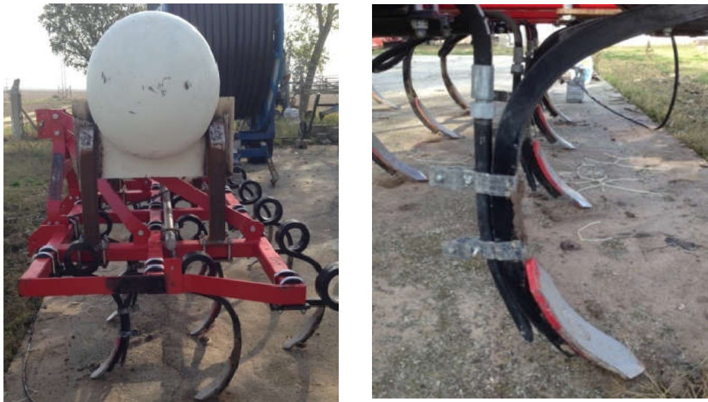
Figure 4. Traditional knife applicator
