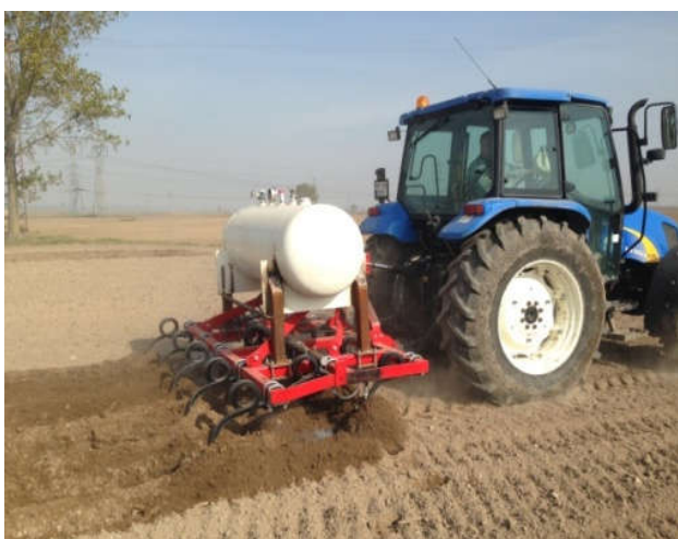
Figure 6. Anhydrous ammonia application
