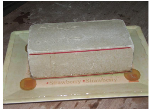
Figure 2. Testing device of absorption by capillarity photographs
