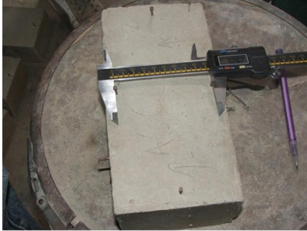
Figure 3. Photographs showing the dimensional variations measurement device
