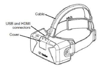
3. Connect the head set cable to the computer CPU: The head set cable has two connecters one is HDMI and the other is USB. Plug both the connectors to the computer.
