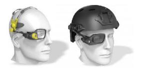
**2.The device (having sensors):-** This device is embedded with the objects like VR helmets, goggles or data gloves with the sensors attached to it for sensing the information of the real objects according to their geometrical relationships. These devices include sensors, Receptors, GPS, Electronic papers, Intelligent Bricks. (https://www.lri.fr/~mackay/pdffiles/AVI98.AugmentedReality)
