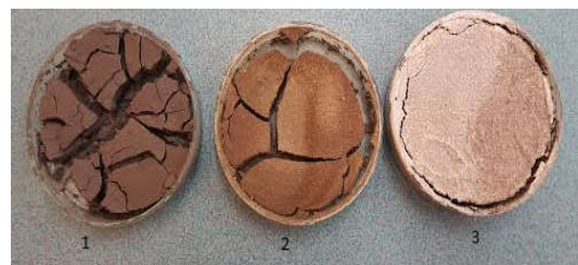
Fig.9. Shrinkage behavior with (1) expansive soil, (2) +10% CHA and (3) +25% CHA
