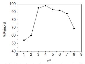
Figure 1. Graph showing the effect of pH on the sorption of Pb(II) ions aqueous solution using Corn husk. Initial lead concentration (100 mg/L).0.5g dry weight biomass with25 mL of Pb (II) Solution
