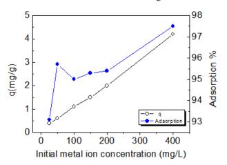
Figure 2. Effect of initial metal ion concentration on biosorption of Pb (II) ions aqueous solution using Cornhusk. 0.5g dry weight biomass with25 mL of Pb (II) Solution. pH4
