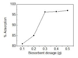
Figure 4.Effect of adsorbent dose for the adsorption of Pb (II) ions onto Corn husk. 100 mg/L lead concentration
