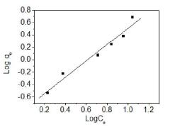
Figure 6: Freundlich isotherm for sorption of Pb (II) ion by Corn husk. 0.5g dry weightbiomass with25 mL of Pb (II) Solution.pH4
