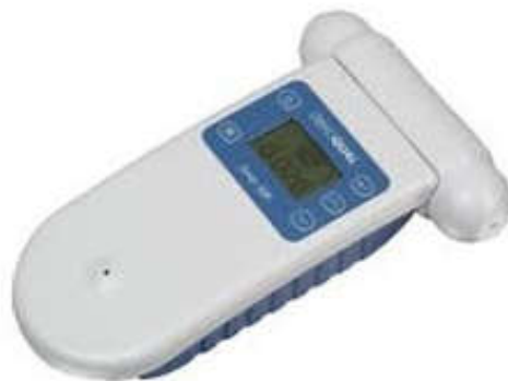
Figure 2. Aeroqual S500 Gas sensitive sensor
