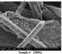
Figure: 9. SEM image of fracture surface of different sized Arecanut husk samples in Acid hydrolysis Pretreatment
