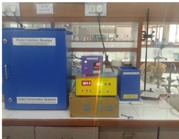
2 hrs run time set in UV-Visible photocatalytic reactor of 450 Watt
